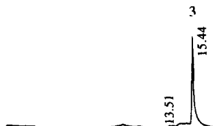
Fig. 7. HPLC printouts showing the rate of conversion of XLC to the reactive vinylsulphone form at pH 8 and the boil. Peak 2 is attributable to XLC-mono-VS; and peak 3 to XLC-di-VS (XLC-VS).
